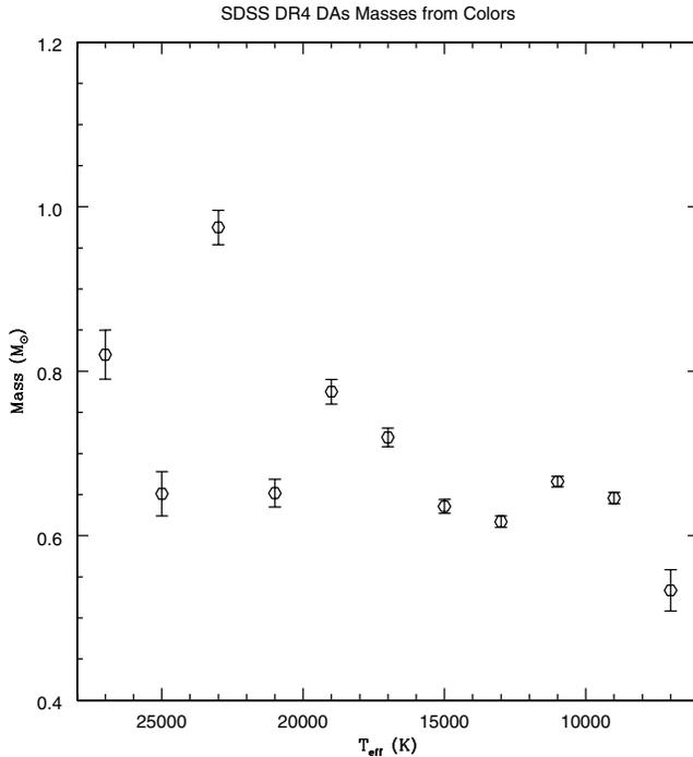
**Figure 4.** Masses for all 7167 DA white dwarf stars derived comparing only the SDSS colours ( $u - g$ ) and ( $g - r$ ) with those predicted from the atmospheric models. For  $T_{\text{eff}} \geq 20\,000$  K and  $T_{\text{eff}} \leq 9000$  K, the colours are degenerate in mass.
